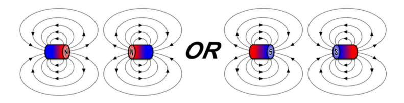
It's only when you hold unlike-poles together (a north pointing to a south) that magnets stick together (they are attracted). Now, the magnetic field acts like a stretched rubber band pulling the magnets together.
